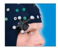
The head reference tool can be attached to an electrode cap easily and tracks all head movements during the navigation session.
