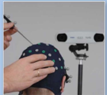
Xensor system setup with 3D Vicra camera
